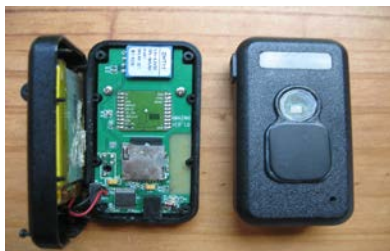
Fig. 2. The custom designed GPS data logger.
